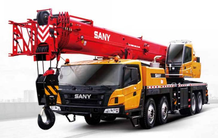
Maximum rated lifting capacity: 70 t Max. Boom Length: 46 m Max. Lifting Height: 62.5 m
